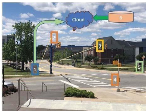
1. Local Server 2. IP camera and traffic controller 3. Traffic signage 4. Local sensor 5. Local sensor 6. Main Server
