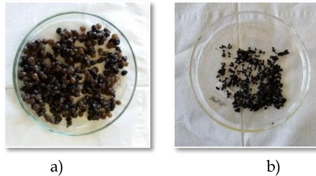
Figure 2. Morphology of the adsorbent, a) wet Ca-Alg/Fe 3 O 4 adsorbent, b) dried Ca-Alg/Fe 3 O 4 adsorbent
