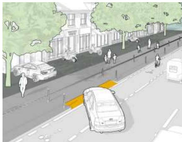
Figure 2 - Illustration of a sidewalk along a lot with parking edges The effective width of the pedestrian lane based on the needs of two wheelchair users passing each other or two adults with goods passing each other is at least is 185 cm.
