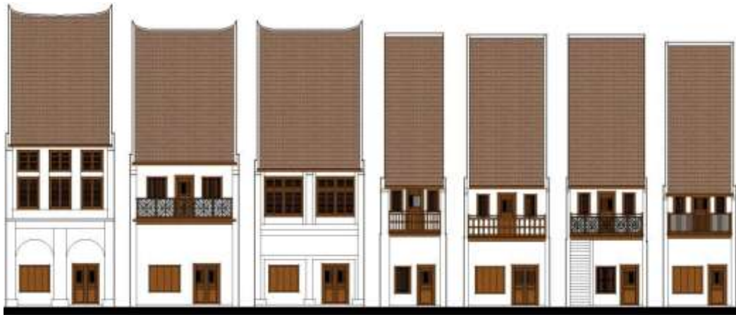
Figure 8: Facade of Malabero Chinese shop house Period 1
