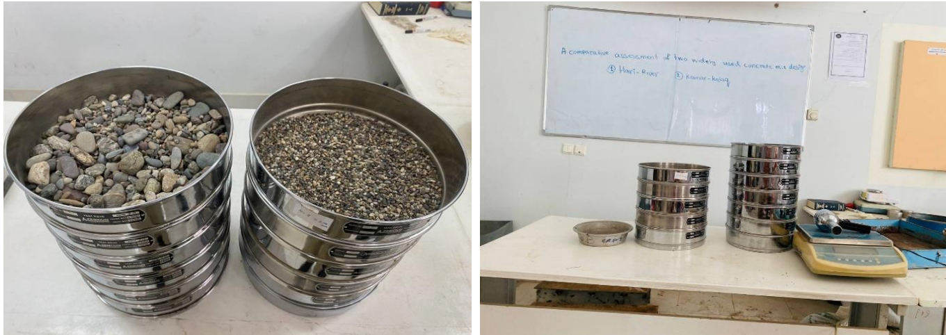
Figure 2. Depicting the equipment utilized in the sieve analysis procedure.
