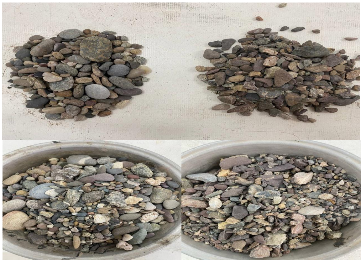
Figure 12. Shows comparison of aggregate shapes between Kamar-Kalaq (right) and Hari-River (left) after sieving
