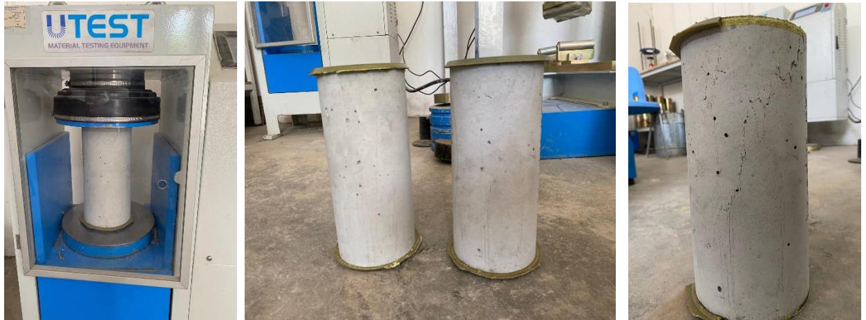
Figure 4 .Representation of a concrete cylinder with caps on both ends, both before and after undergoing compression testing.
