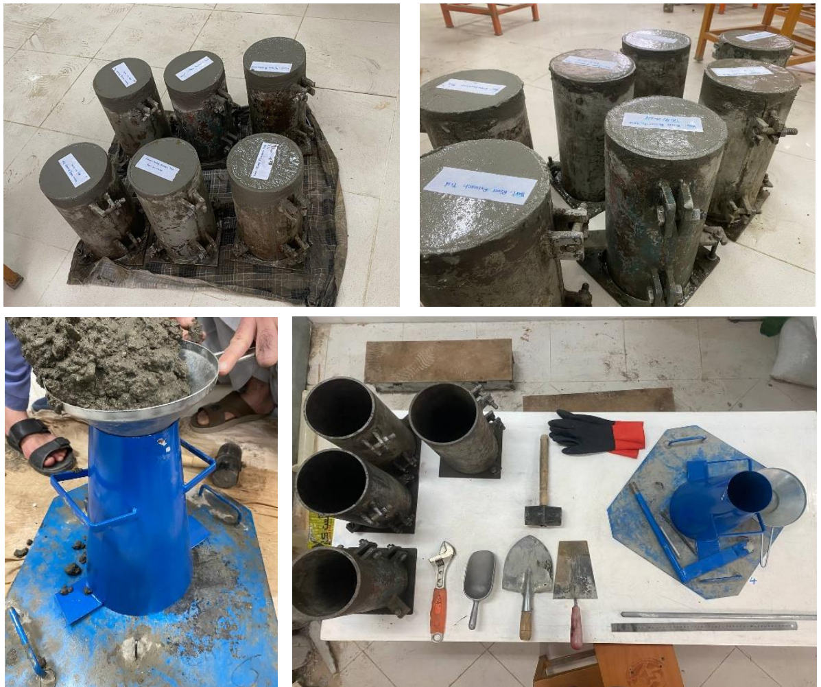
Figure 3. showing slump pouring process with cylinder mold and accompanying materials for concrete casting
