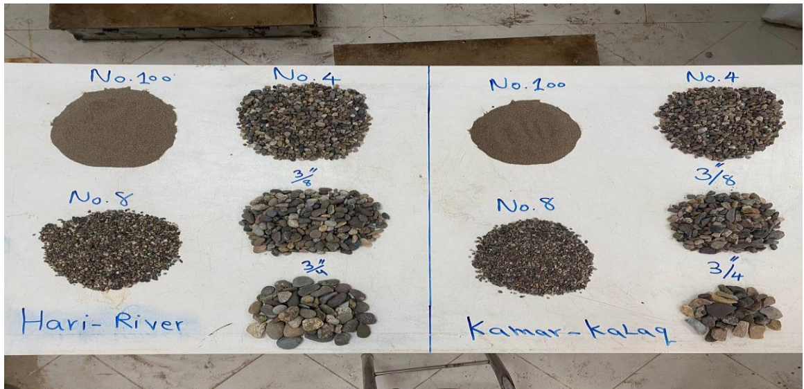
Figure 11. Shows comparison of aggregate shapes between Kamar-Kalaq (right) and Hari-River (left) after sieving
